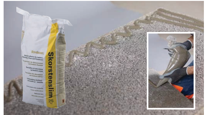
Mix jointing adhesive as per instructions on the bag. Apply 15-20mm beads using the supplied application bag as shown in the picture above.
